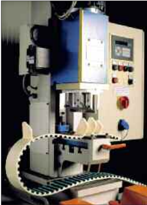
Cleat welding machine
